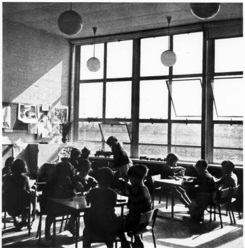
2, one of the handcraft rooms under construction. 3, the covered way outside the assembly hall. 4, a section through a typical external classroom wall. 5 and 6, outside and inside the infants' classroom block. Here the standard window shown in 4 has one pane added to allow the smaller children to see outside. The walls are of fair-faced brickwork, distempred.
