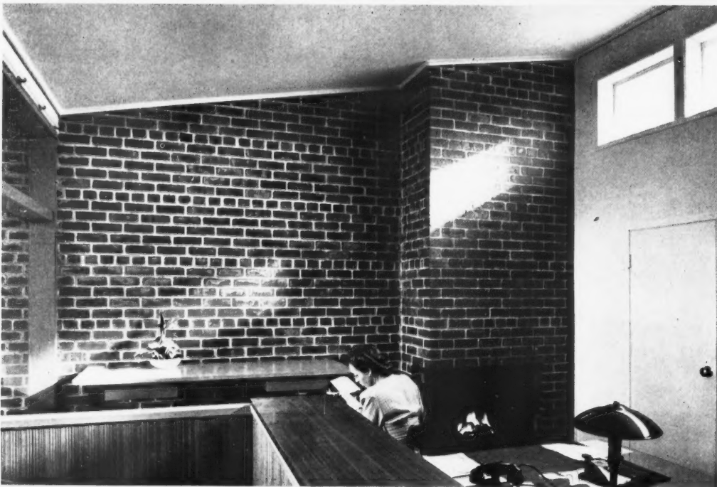
14, the office and enquiry desk. The right-hand wall and the ceiling are faced with plasterboard.
